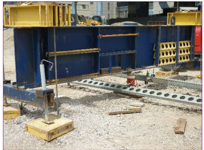
Figure 6: Modulus test set-up.
